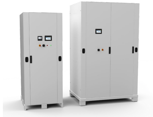
Figure 5: REGATRON's liquid-cooled system solutions up to IP54 with various power levels e.g. 54...162 kW (left) and 216...324 kW (right). The remote control unit RCU, indicator lights, emergency stop button, and main switch allow the user to operate the system on the enclosure's front door.
